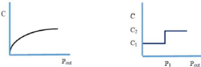
(a) Continuous-state channel      (b) Two-state channel
