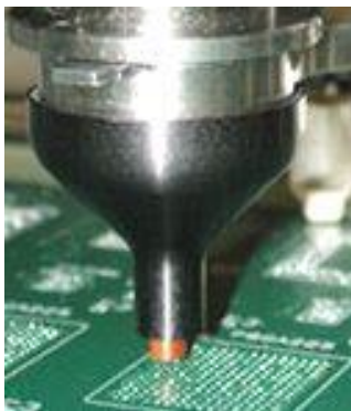
Figure 6.3: BGA site vacuum system.
