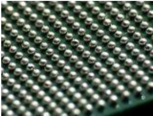
Fig.6.2: Large Scale BGA Component Rework
