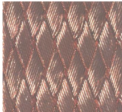
Figure. 5.3: Close up of copper solder wick
