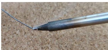
Fig.5.15: Tinning Solder Iron Tip
