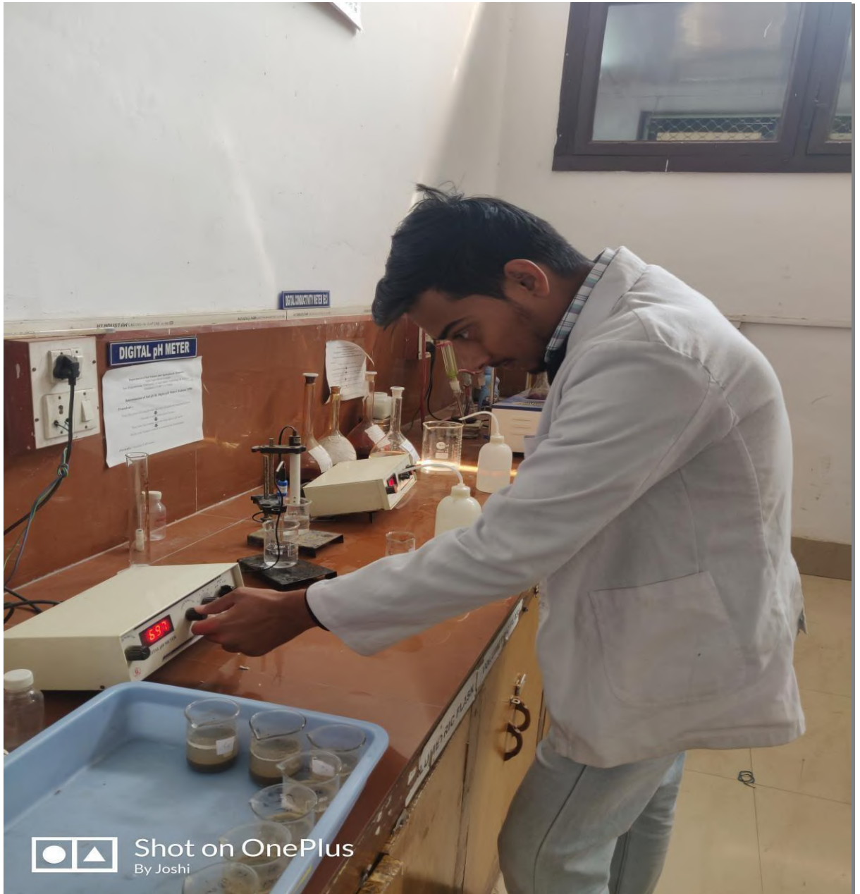
Plate No.3 Analysis of soil pH and EC by digital pH and digital EC meter
