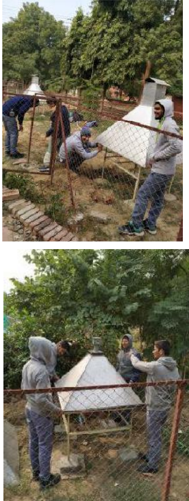
Figure 5 Undergraduates setting up DEASA detectors in the field.
