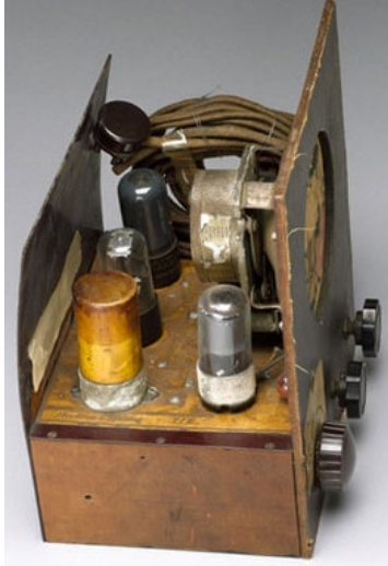
Fig. 1.5 Radio made by Paul Eisler that Uses first printed circuit board (PCB)
