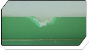
Fig 8.16(a): Damaged PCB edge
